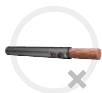
Damaged conductor insulation
