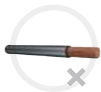
Too less twisted single wires
