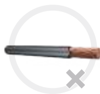
Insulation not cut in properly
